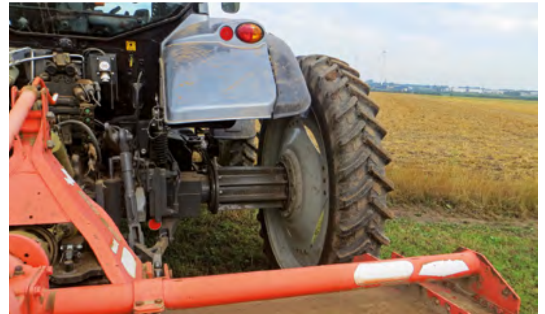
Using wheel spacers the N143 has 3,20 meter wheel track.
