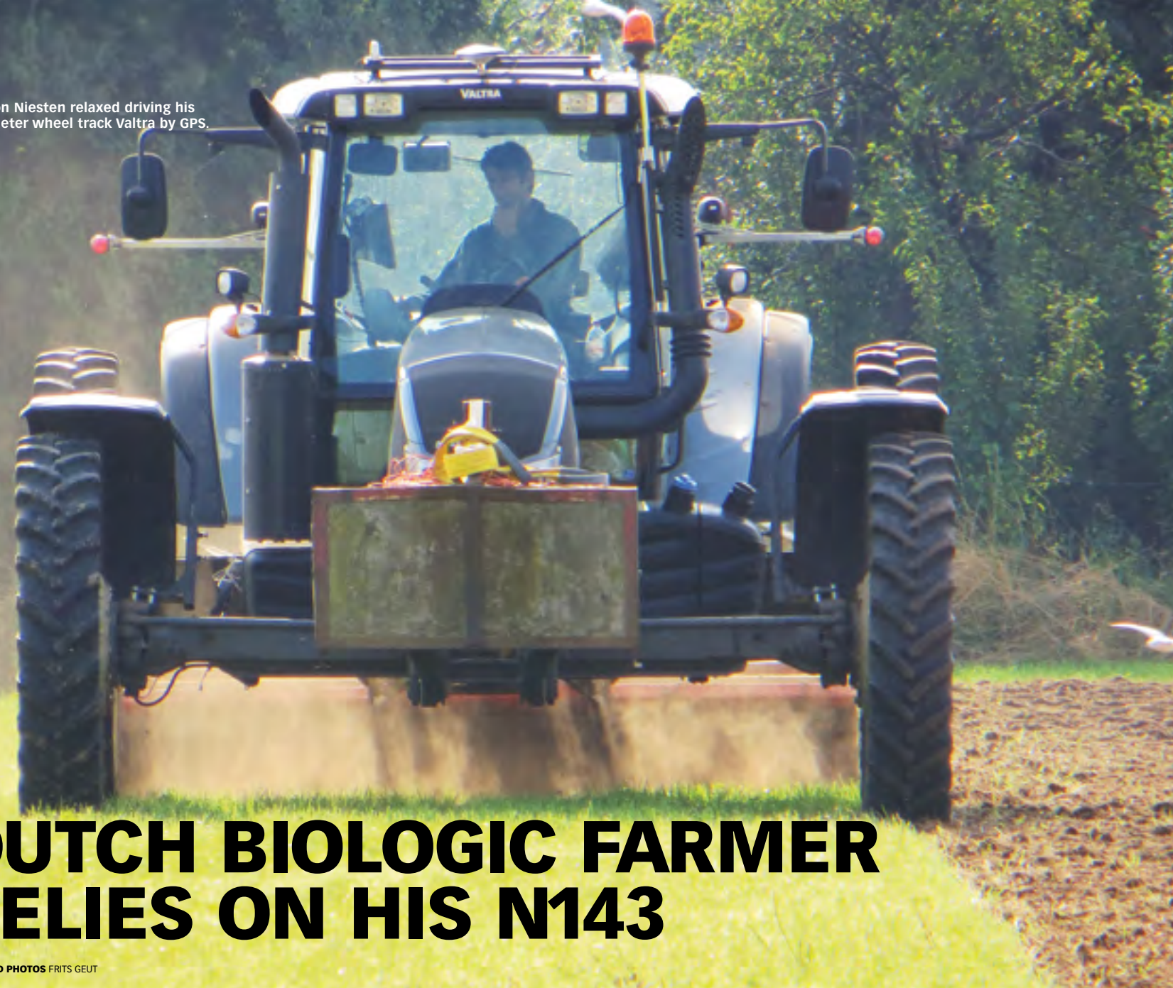
Using wheel spacers the N143 has 3,20 meter wheel track.
